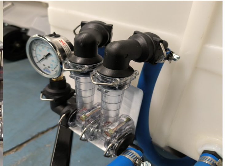
Figure 4: Flow monitor and pressure gauge
