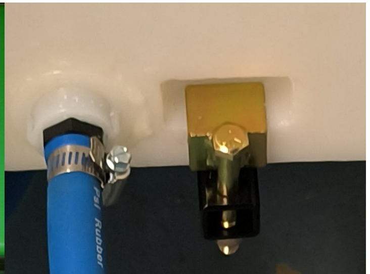
Figure 6: Mount tank and secure with tank locks
