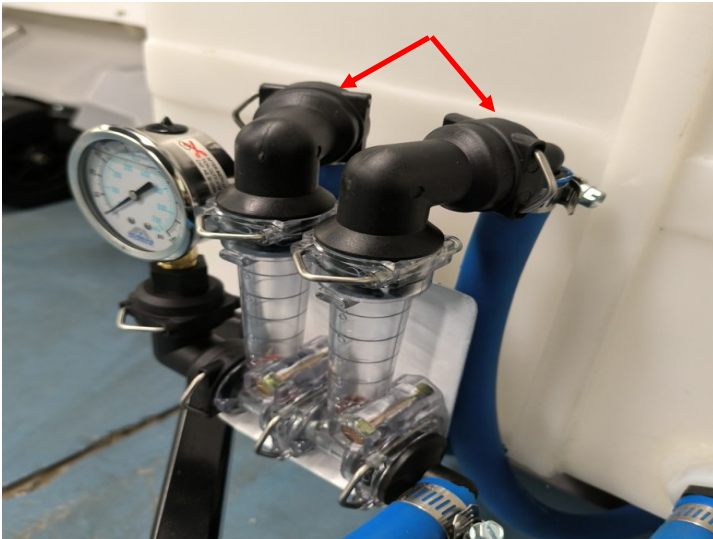
Figure 9: Attaching nozzle feed hose to flow monitor
